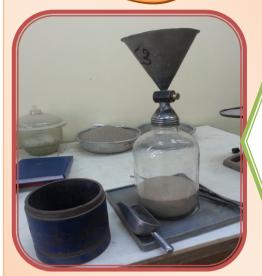
Several density field Which contain and suppress the bottle and a glass plate and metal mold density
