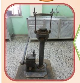
Jack Hyderoleik Which is used for the extraction of soil samples from templates.
