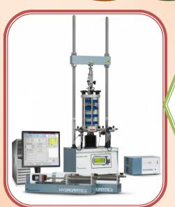
Triaxial test is developed that can automatically bring up to 6 full and independent tests at the same time, from the beginning to the end system,
