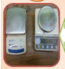
**Sensitive electronic** balance Which is the weight of the soil and is available in different sensitivities (1 gm., 0.1gm, 0.01gm)
