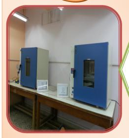
ELE soil type drying oven Which drained soil and can be a temperature through an electronic control panel
