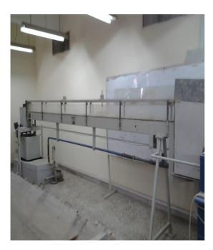
**4-Hydraulics bench:**To measure the volume flow rate (discharge).
