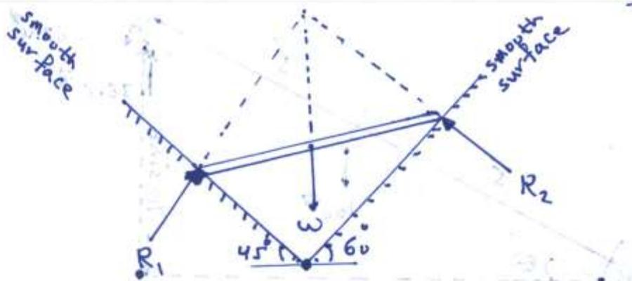
Q: The uniform bar AB is  $10$  long and weighs  $100\text{ N}$ . Find the angle  $\theta$  at which the bar will be in equilibrium.
