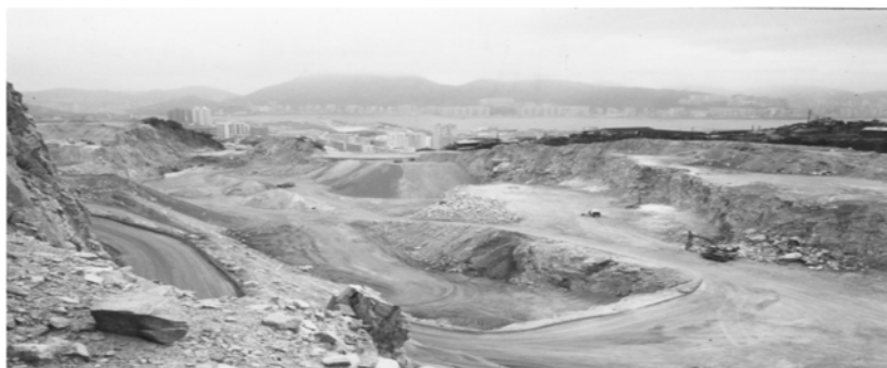
Fig. (6.5). Quarrying granite for aggregate, Hong Kong.
