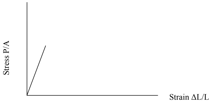
Stress – Strain curve for non ductile material – Cast iron (no plastic deformation)
